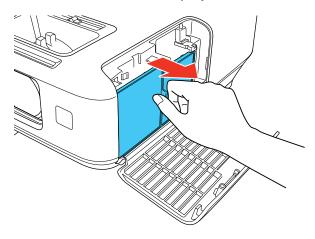
**Note:** Air filters contain ABS resin and polyurethane foam. Dispose of used air filters according to local regulations.
